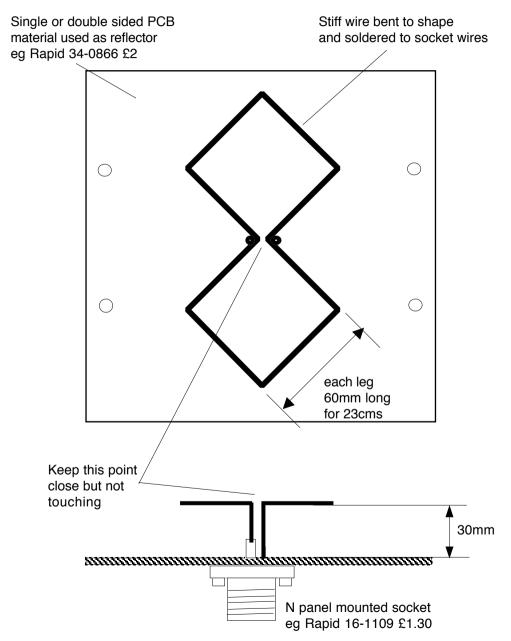
Antenna could be waterproofed in a graphite free (non black) sandwich box etc
